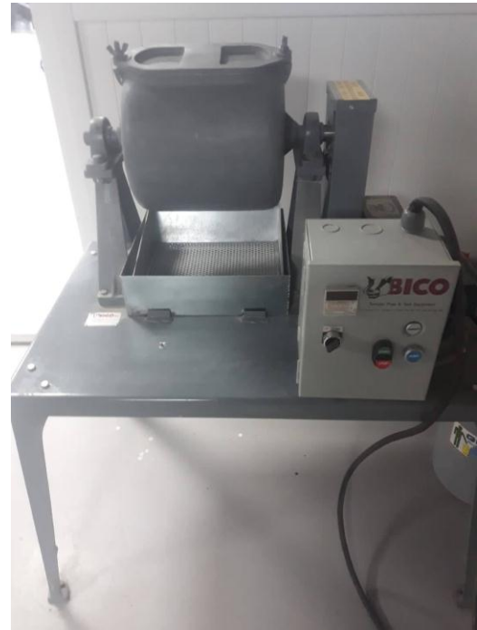
Picture 1 F.C.BOND BALL MILL
